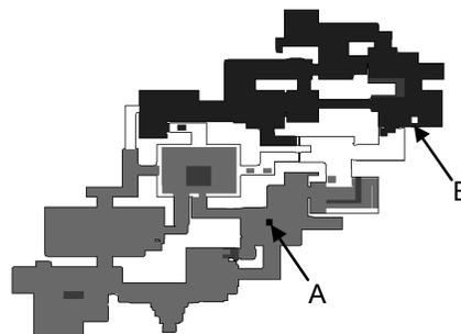
Figure 1. Example from a simulation of the use of frontiers within the online multi-participant game Quake II. If A stays in the light grey region and B stay in the dark grey region then they never have to send a network packet to each other because they can never see each other.
